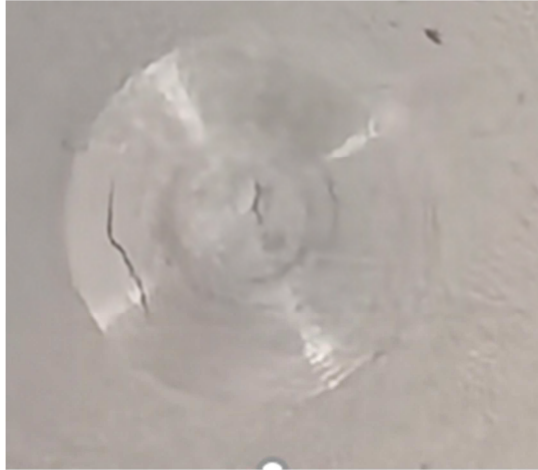
Figure 12. RSW cracks.
