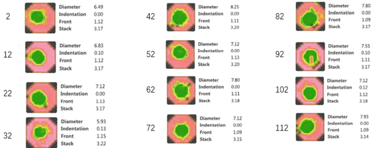
Figure 24. Ultrasonic inspection of spot welding points (Process Parameter 2).
